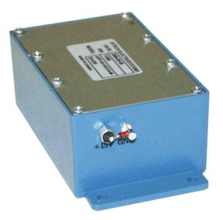
The +15V input terminal is protected with a 1N4746A Zener diode, which will fail as a short if an excessive positive voltage (> 18V), or a negative voltage, is applied to the terminal.
